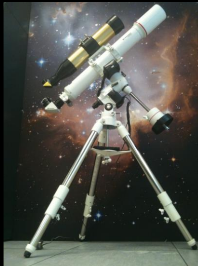
2 sets of 9cm H \alpha and 10cm white light telescopes at ESAC
