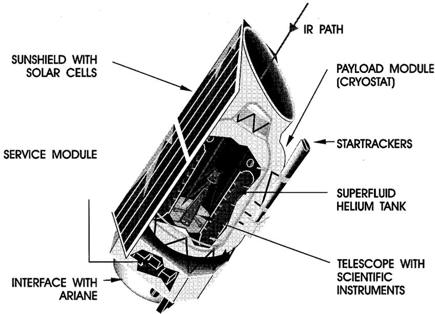
Fig. 1. A cut-away schematic of the ISO satellite
