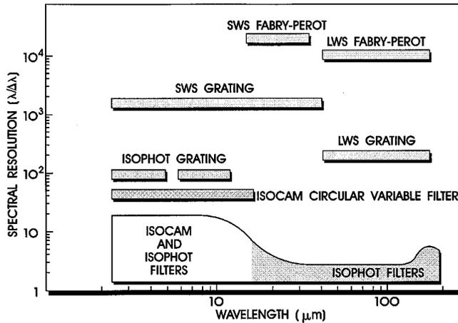
Fig. 2. Photometric and spectroscopic capabilities of ISO.
