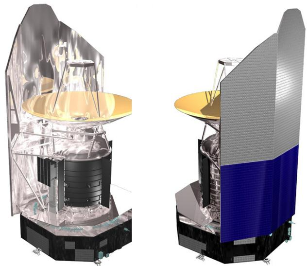
Figure 1. Current Herschel configuration, towards the end of phase B. It measures approximately 7.5 m in height, 4 m in width, and has launch mass of order 3170 kg. (Courtesy and all rights reserved Alcatel Space Industries)
