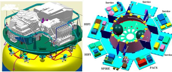
Figure 3. On the left the accommodation of the FPU's of science payload in the cryostat on the optical bench, clockwise from the left PACS, SPIRE, and HIFI. On the right the 'warm' electronics inside the service module. (Courtesy and all rights reserved Astrium-ED (left) and Alenia Spazio (right))
